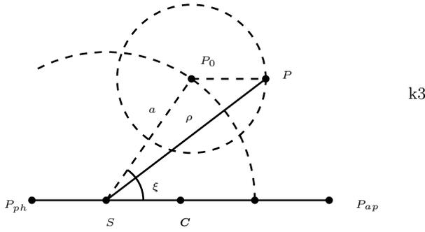
Fig. (k3): The first attempt to establish the law  $\rho \dot{\xi} = \text{const}$ . Eccentricity ( $e = 0.4$ ) is much larger than the real value, for illustration purposes. The deferent is a circle of radius  $a$  around  $S$  and the epicycle of radius  $ea$  is centered at  $P_0$ , with anomaly  $\xi$  with respect to  $S$ , the planet is in  $P$
