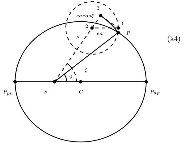
Fig. (k4): Kepler’s construction of the ellipse. The eccentricity is  $e = 0.4$  to make a clearer drawing. The planet is in  $P$ . The segment  $23$  is the projection on  $S3$  of the segment  $31$  and the segment  $SP$  is equal to  $S3$ . The epicycle (dashed circle) is no longer holding the planet but it determines its position. The anomaly  $\xi$  is the anomaly of the center of the epicycle. Motion verifies the law  $\rho \dot{\xi} = \text{const}$ .
