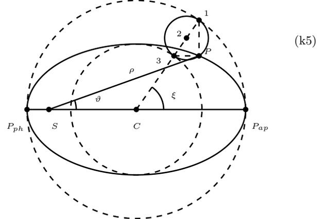
Fig. (k5): Fabricius’ interpretation, see<sup>3</sup> p. 402-403, of Kepler’s ellipse. The ellipse has very high eccentricity ( $e = 0.8!$ ) to make visible the small epicycle. The planet is in  $P$  and  $C3 = b$ ,  $C1 = a$  and the center of the epicycle is  $2$ . Eccentric anomaly reckoned at  $C$  and the angle  $12P$  is  $2\xi$
